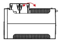
3. Aligned all arrows marks and slide the battery compartment cover back onto the battery housing. Double check if battery compartment is well-locked.
